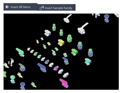
• **Size Import:** Imports all sizes of a component family into the current drawing. The spacing settings are requested dynamically when executing the command to ensure maximum flexibility.
