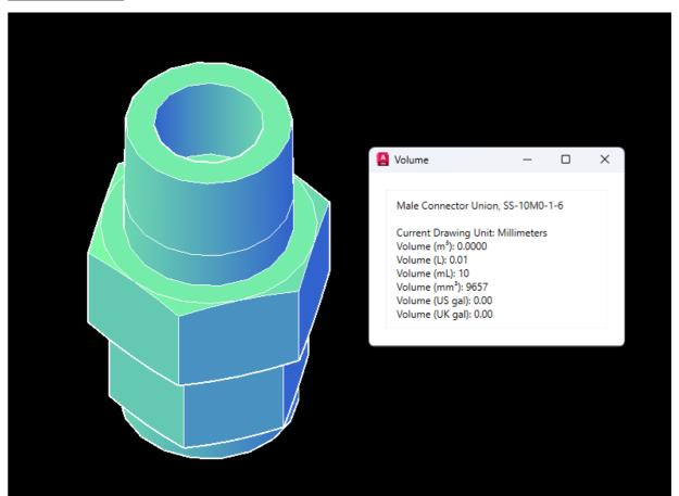
• Object Properties: Displays detailed object-specific properties.
